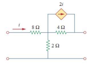
7-b. For the ladder network in Fig, determine the h parameters in the s domain. 10 (CO4)
